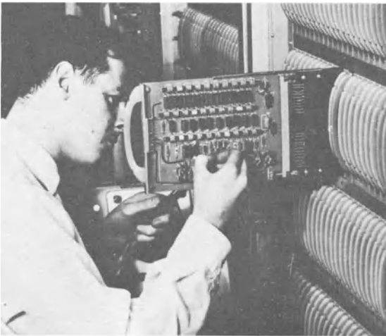
Figure 27.8. Testing and replacing a logic circuit
