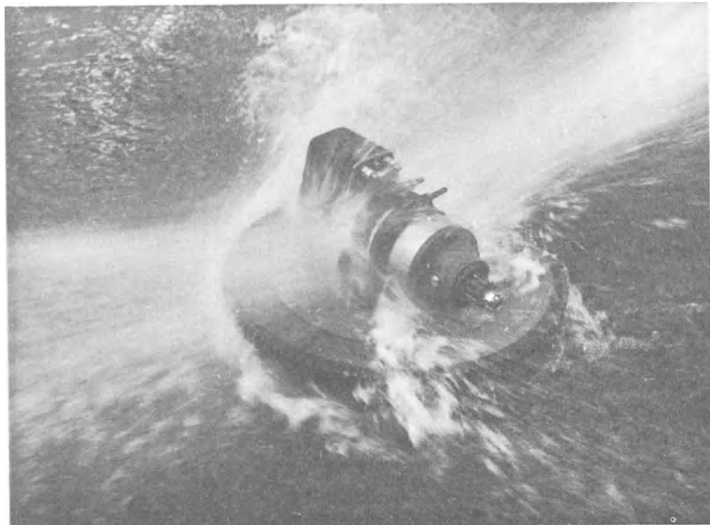
Figure 24.5. Two views of a starter subjected to water from a fire hose, to simulate the effect of wheel splash at 90 m.p.h.
