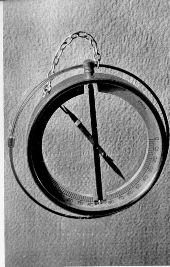
Short and Mason miner's compass; indicates direction of ore. Taylor Instrument Companies, U.S.A. Photo: Museum of Modern Art, New York.
