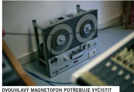
DVOUHLAVÝ MAGNETOFON POTŘEBUJE VYČISTIT
