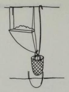
Leonardo da Vinci: apparatus for measuring resistance to traction.
