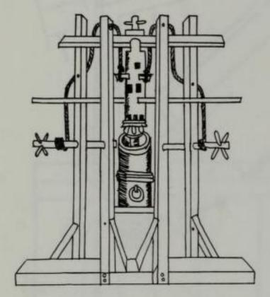
Munich MS: machine for boring cannon.
