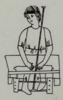
Two-pedal treadle lathe (stained glass at Chartres).
