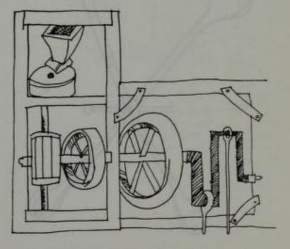
Hussite MS: handmill with rod and crank system.
