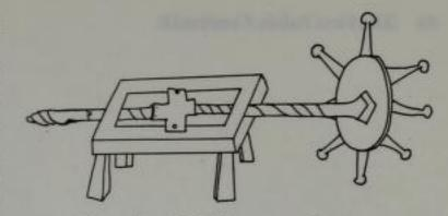
Taccola: machine for hollowing wooden pipes.
