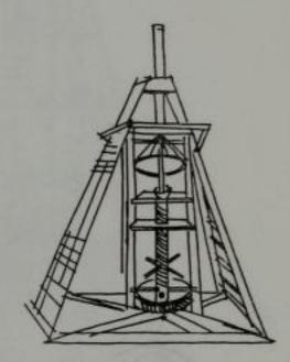
Leonardo da Vinci: drilling machine for wooden beams.
