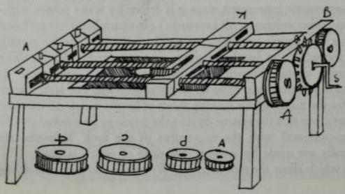
abrasive matter. Leonardo conceived of machines differing slightly from one another, for polishing mirrors with concave surfaces, according to the radius of curvature and according to the focal distance. The same crank turns, on two different planes, the surface to be polished and the mill. For Leonardo a good concave spherical mirror had to have a focal distance of F8. These mirrors were made during his time in Rome when Leonardo was studying the formation of images.
