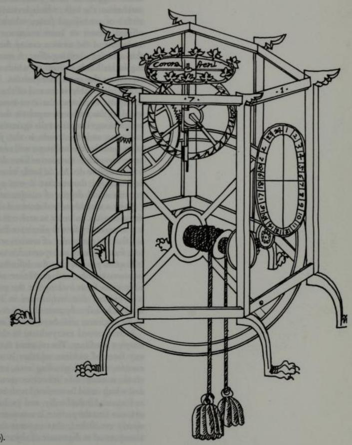
Dondi: Clockwork mechanism (1340).
