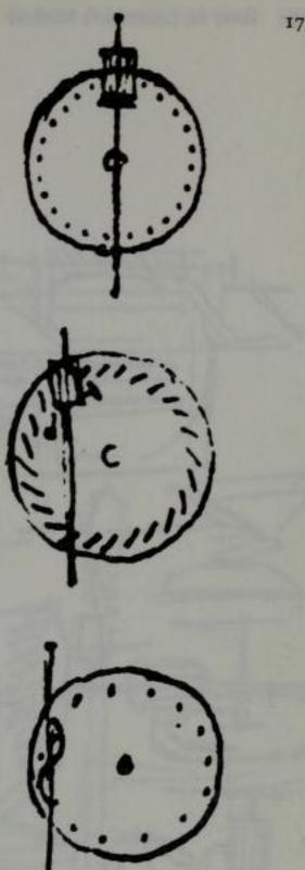
Alignment of pinion axis in relation to the centre of the toothed-wheel and the effects of wear. Drawing by Leonardo da Vinci.
