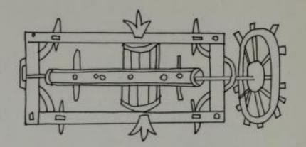
Hussite MS: machine for hollowing wooden pipes.
