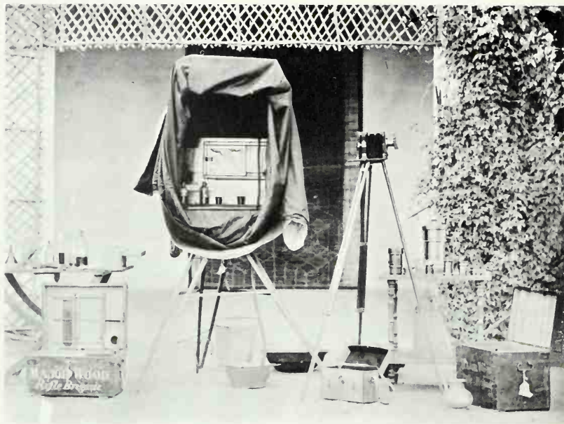
Colonel Henry Wood: His chemicals, dark tent for sensitising and developing plates, baths, camera and tripod, lenses and cases – the kind of equipment Bourne was using in India at much the same time.
