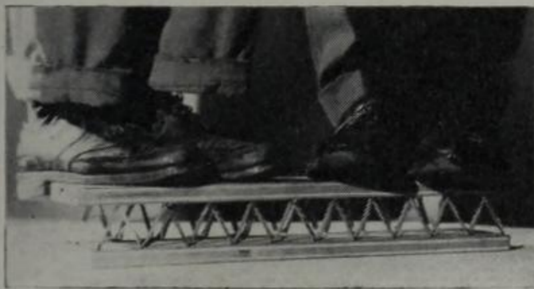
Fig. 71. O Arthur Kersten, 1940 Expanded metal structure In spite of the thin gauge metal this structure carries 600 lbs
