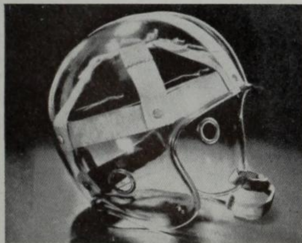
Fig. 35. Football helmet, 1939 Structural application of the eggshell principle. Though relatively thin, the helmet achieves great strength. For easier discrimination of the different playing groups, the inside of the helmet can be sprayed with color, with the double advantage of keeping the outside surface glossy and protecting the paint against abrasion
