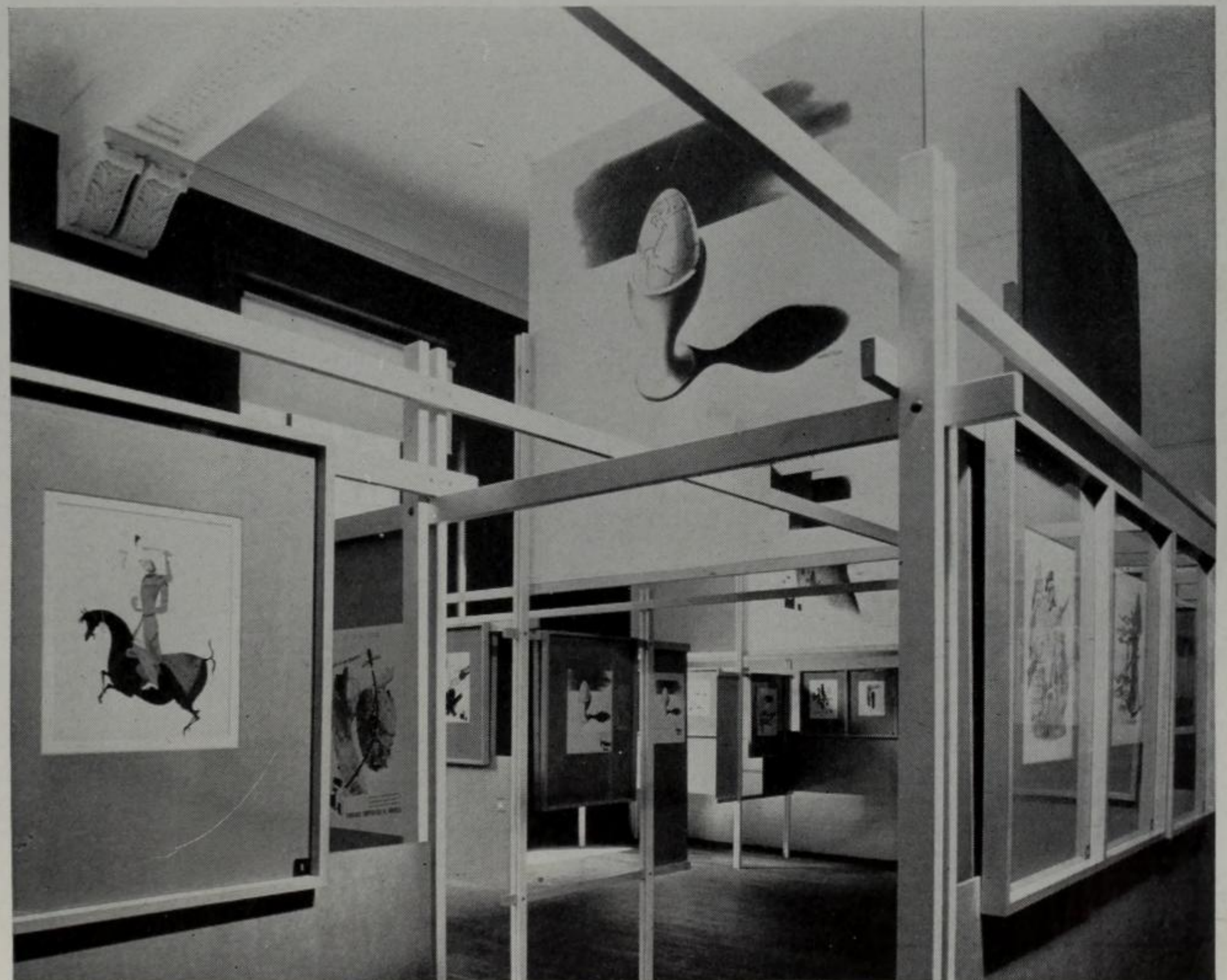
Fig. 370. Herbert Bayer, 1945 The exhibition of the Container Corporation of America for modern advertising The structure was designed as a knock-down solution for easy packing, transportation and assembly
