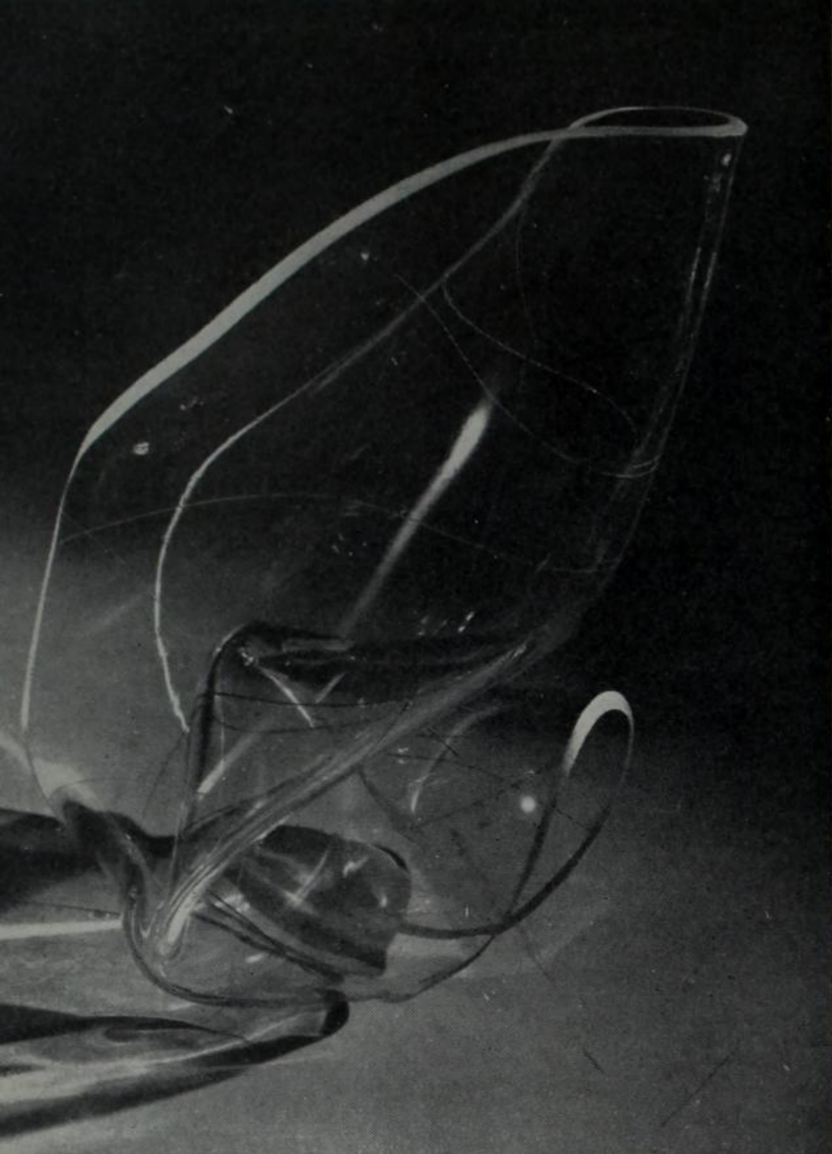
Fig. 61. ○ L. Moholy-Nagy, 1940 Convex-concave Circular disk of transparent material, twisted and warped to demonstrate greater resistance against pressure
