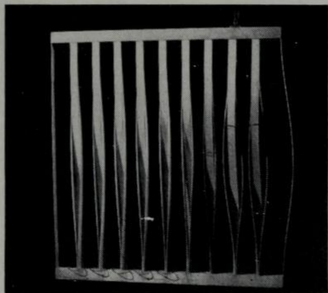
Fig. 78. O Elic Nekimkin Elastic wall This structure originated through experiments with new plywood joints. The construction of the single elements can be seen in closeup in the illustration at the right
