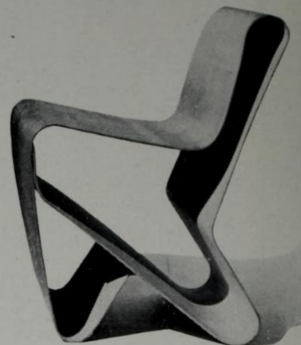
Fig. 94. O Nathan Lerner, 1940 One piece chair This chair is made of a single sheet of \frac{3}{8} " plywood bent into shape without waste, using only two lap joints. This construction produces a springy chair without upholstery; it may however be upholstered by affixing an airfoam pad, covered with fabric, to the seat and back
