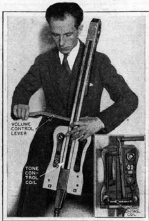
The electrical unit which controls the tone and volume of this stringless cello is contained in the sound box.
