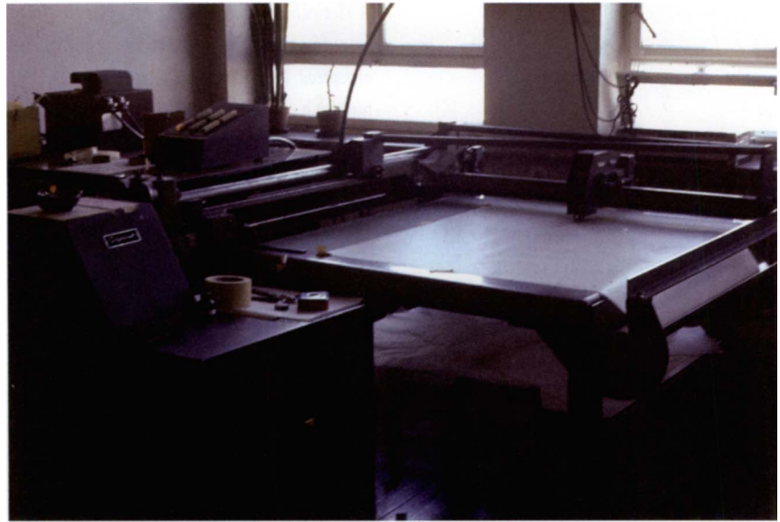
The Zuse Graphomat Z64 drawing machine, at the Computing Center, University of Stuttgart, 1965. The drawing area was about 4 feet square (1.2 x 1.2 m). (Photograph © the author)
