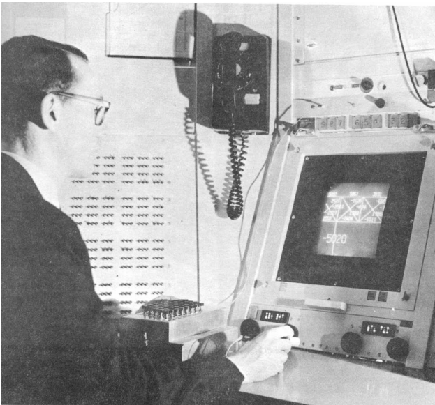
SketchPad in use. On the display part of a bridge. Ivan Sutherland is holding the Light pen. The push buttons used to control specific drawing functions are on the box in front of the author. Part of the bank of toggle switches can be seen behind the author. The size and position of the part of the total picture seen on the display is obtained through the four black knobs just above the tabl
