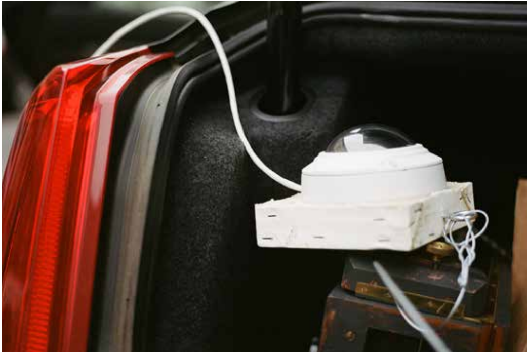
The eye of Wordcar was an Axis M3007 surveillance camera
