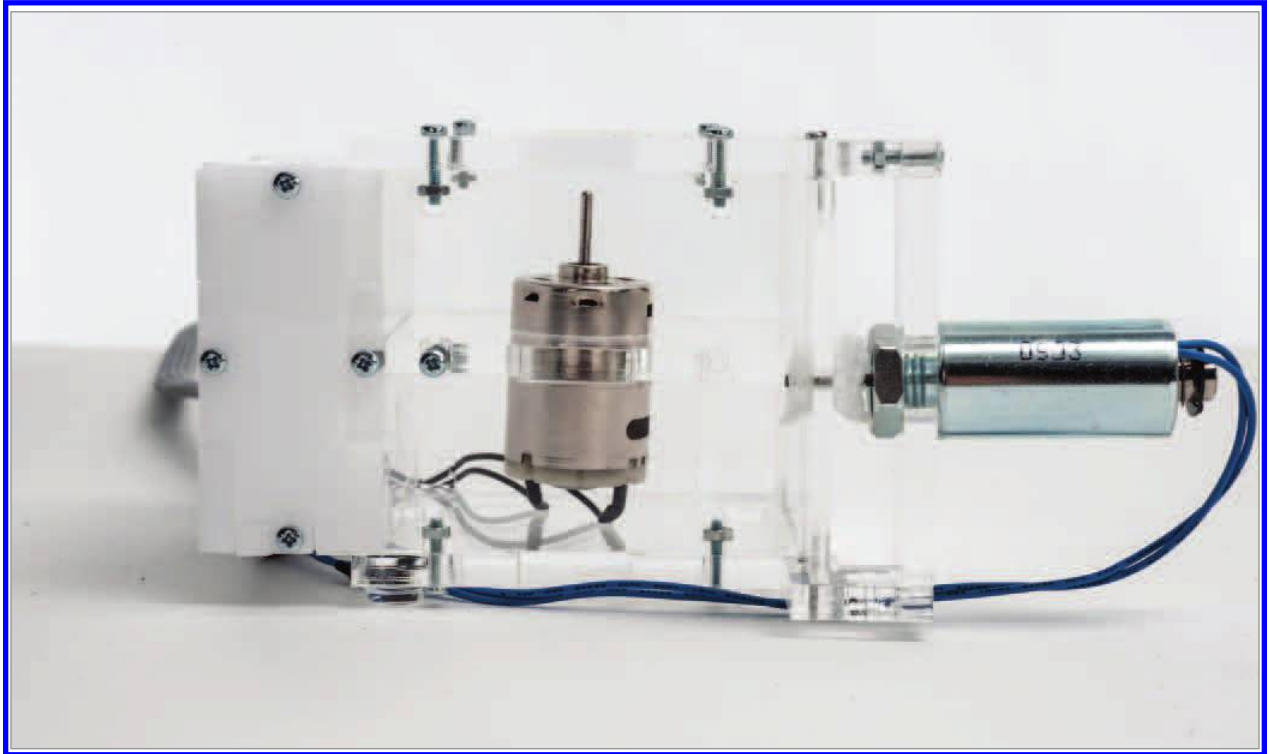
Fig. 3. Mo H. Zareei, Motor , mechatronic sound-sculpture, electronics, metal, plastic (transparent enclosure dimensions: 8 x 8 x 10 cm), 2014. The noise of the DC motor is modulated using a solenoid-actuated pivoting door. (© Mo H. Zareei)
