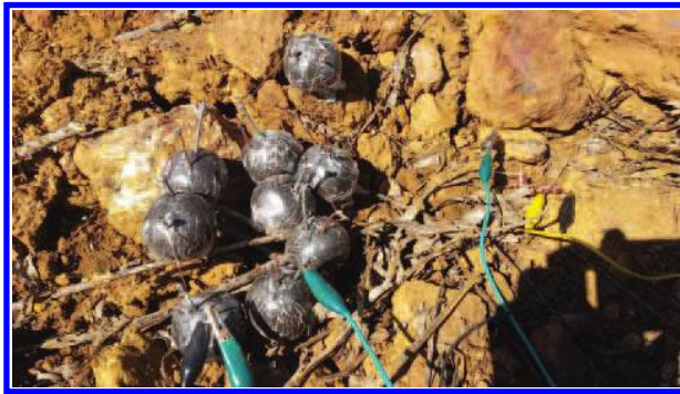
Fig. 6. Ryan Jordan, derelict electronics workshop, 2014. Crystal amplifier powered by clay battery using iron pyrite deposits in the earth at Oficinas do Convento, Portugal. (Photo © Ryan Jordan)
