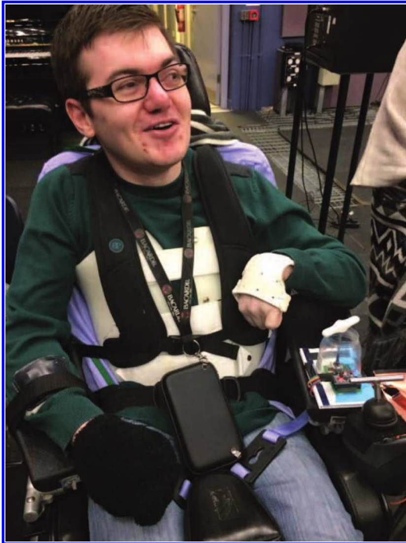
Fig. 4. Ruben and his joystick Arduino interface, 27 March 2015. The interaction mode was designed to be similar to his assisted control wheelchair system. (Photo © Cathryn Hogg)
