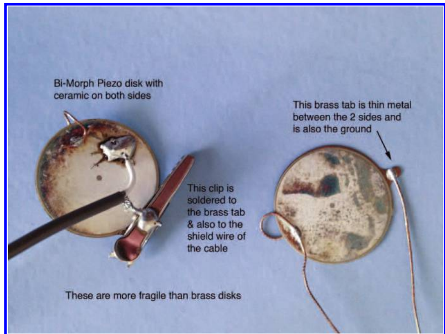
Fig. 6. Richard Lerman, bi-morph piezo. The author has used more than 100 different types of piezo disks, such as this one, in his work in the field over the years. (Photo: © Richard Lerman)
