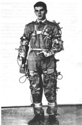
FIGURE 8.—An unpowered exoskeleton built by Cornell Aeronautical Laboratory under Department of Defense contracts. Actuators are not simulated. The exoskeleton would be a "man amplifier." (Courtesy of Cornell Aeronautical Laboratory.)
