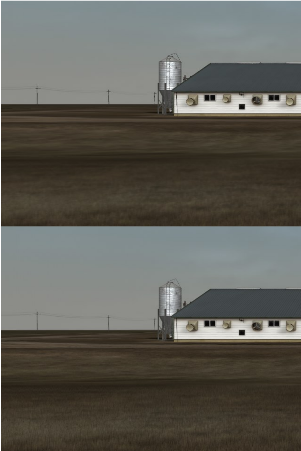
Figure 17. Comparison of frames from two performances of Sow Farm, one with default NVIDIA display driver settings applied (top) and the second with custom NVIDIA display driver settings applied to force multi-sample anti-aliasing and anisotropic texture filtering (bottom).
