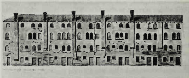
Row-houses from the 15th century in Calle dei Preti near Via Garibaldi in Venice. The façades were probably more uniform originally. Each story had its own rhythm which was repeated with strict regularity across the entire row, the houses being separated by the regularly placed chimneys. Each flat was in two stories, one street-door leading to the dwelling on the lower floors, the other to the one on the two upper floors
