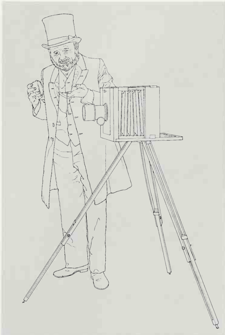
570. Lens Cap. Until the advent of the gelatin dry plate in the 1870s, most exposures were made by removing the lens cap and replacing it after a suitable interval of seconds—or minutes.
