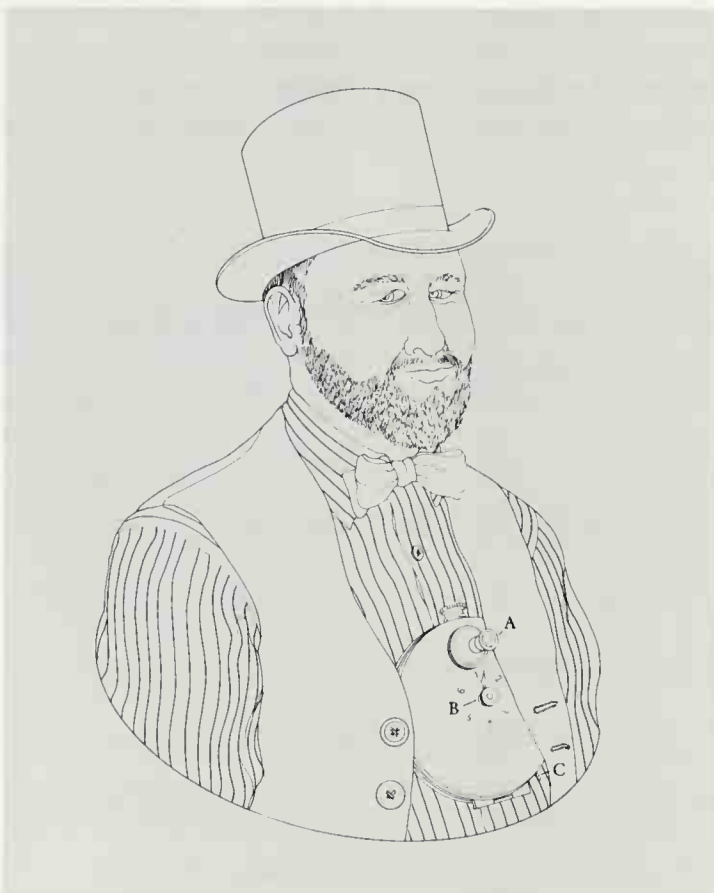
566. Stirn Secret Camera . The Carl P. and Rudolph Stirn Secret or Waistcoat camera of 1886 was worn under a waistcoat, the lens (A) poking through a buttonhole. The circular plate was turned and the shutter set when the pointer (B) was rotated. Exposures were made by pulling on a string (C).
