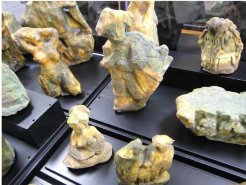
Figure 5. Illustrating digital data by scaled physical models 3D-printed by a rapid prototyping machine
