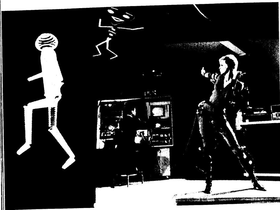
Lee Harrison III photo montage featuring a dancer with body-mounted sensors controlling real-time animation on the ANIMAC (hybrid graphic- animation computer) 1962 Denver
