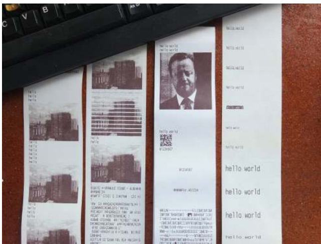
Figure 5: A test print on narrow receipt paper showing text and dithered images from social media. Photography, Brendan Howell, 2018.
