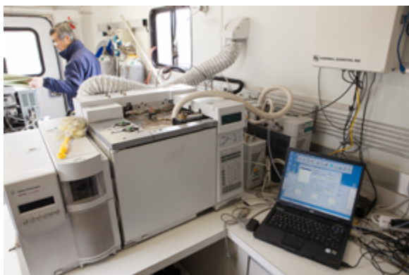
The interior of the Mobile Ambient Air Monitoring Laboratory (MAAML), the most advanced mobile lab of its kind. The Bureau of Pollution Control and Prevention for the City of Houston deploys the MAAML to locations of known air pollution events in order to monitor the industry but also to deter known offenders from repeatedly exceeding federal limits. Despite efforts like this, toxic atmospheric events occur all the time, but accurate source detection is difficult.
