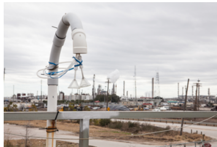
Teflon tubes and glass sampling funnels inhale the atmosphere to collect samples of toxins and particulate matter at the City of Houston's Clinton Drive air monitoring site.
