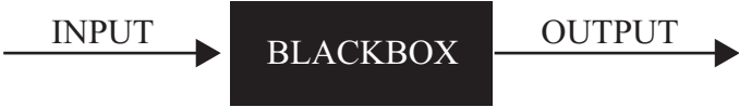
Figure 2.3 A blackboxed system processes input into output without the user’s knowledge of the interior functionality of the object. Image Garnet Hertz.
