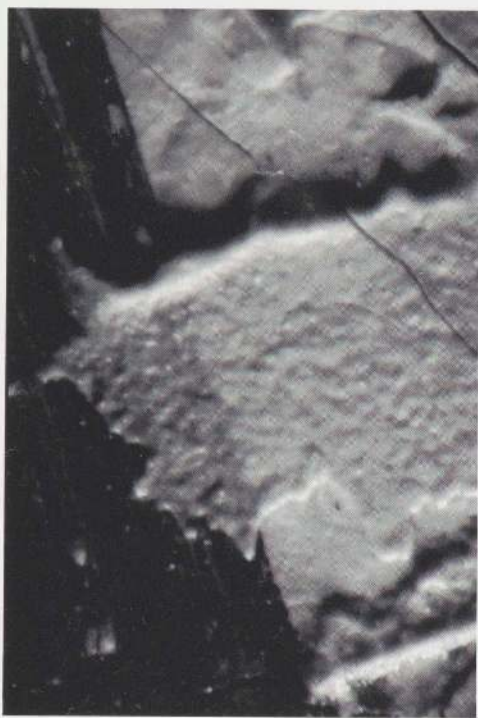
Fig. 1. A translucent white layer has been applied over an opaque white layer.
