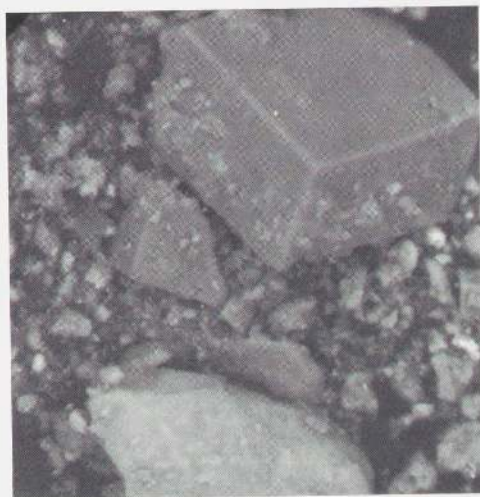
Fig. 3. The numerous small particles are typical-sized calcite particles. The large form in the upper right is also calcite (backscatter electron image).
