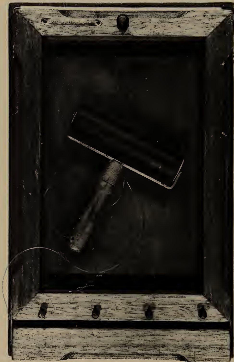
"Pinocchio," a handmade wooden mimeographer.
