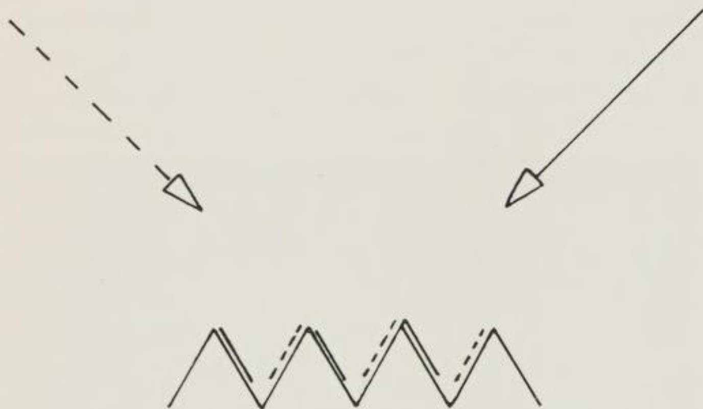
131 b Corrugated card illuminated by two projectors at 180^\circ
