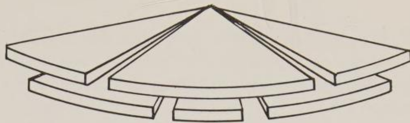
156 Segmented disc, with overlap, detail of construction
