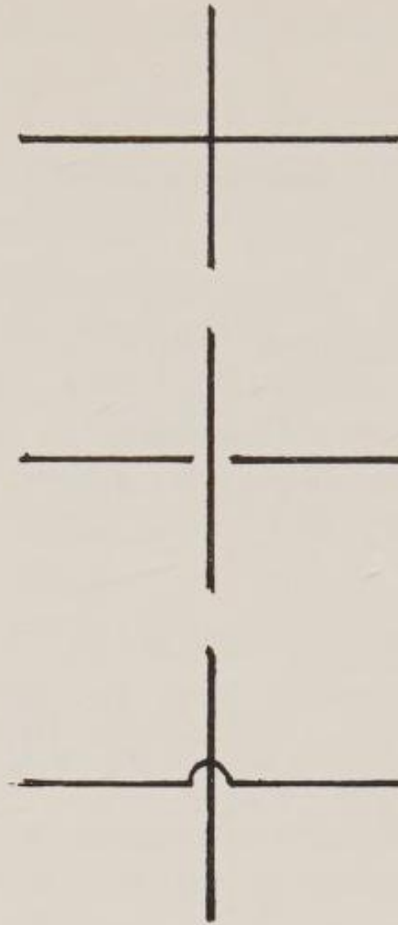
(c) crossing wires
