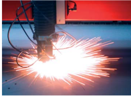
Cutting head of a laser cutting machine plate size: 3 x 1.5 meters, plate thickness: up to 1 centimeter
