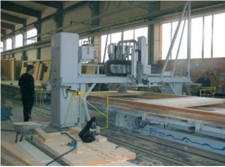
digitales bauen, Volkmar Hovestadt The graphic shows a 30-meter-long machine for molding wood CAAD.ETHZ.CH
