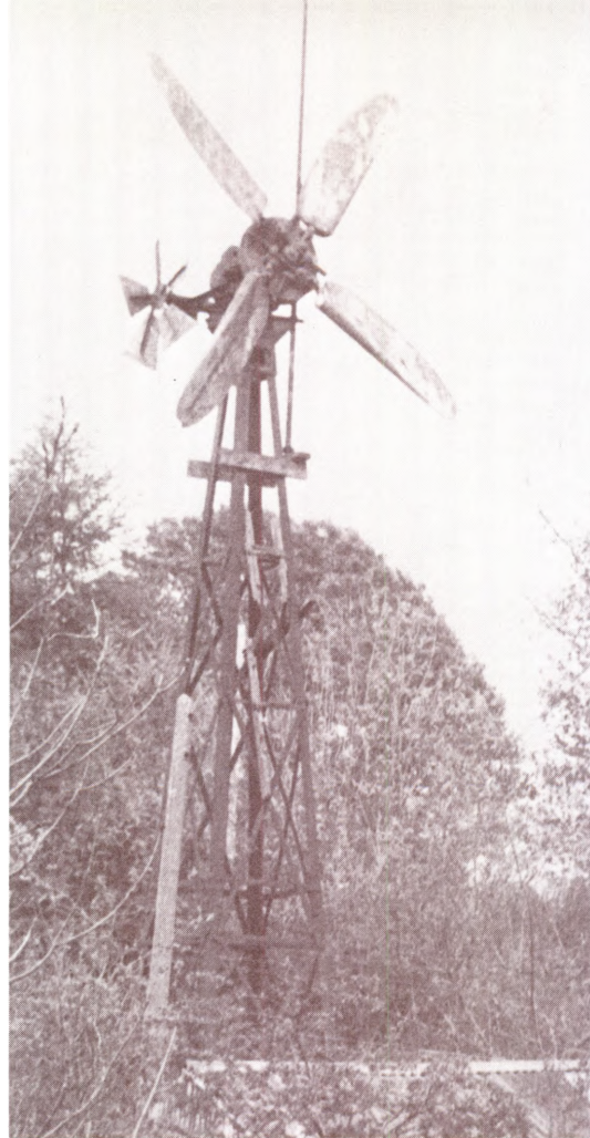
Note: the sophisticated and robust blade feathering mechanism on this old wreck in mid Wales.
