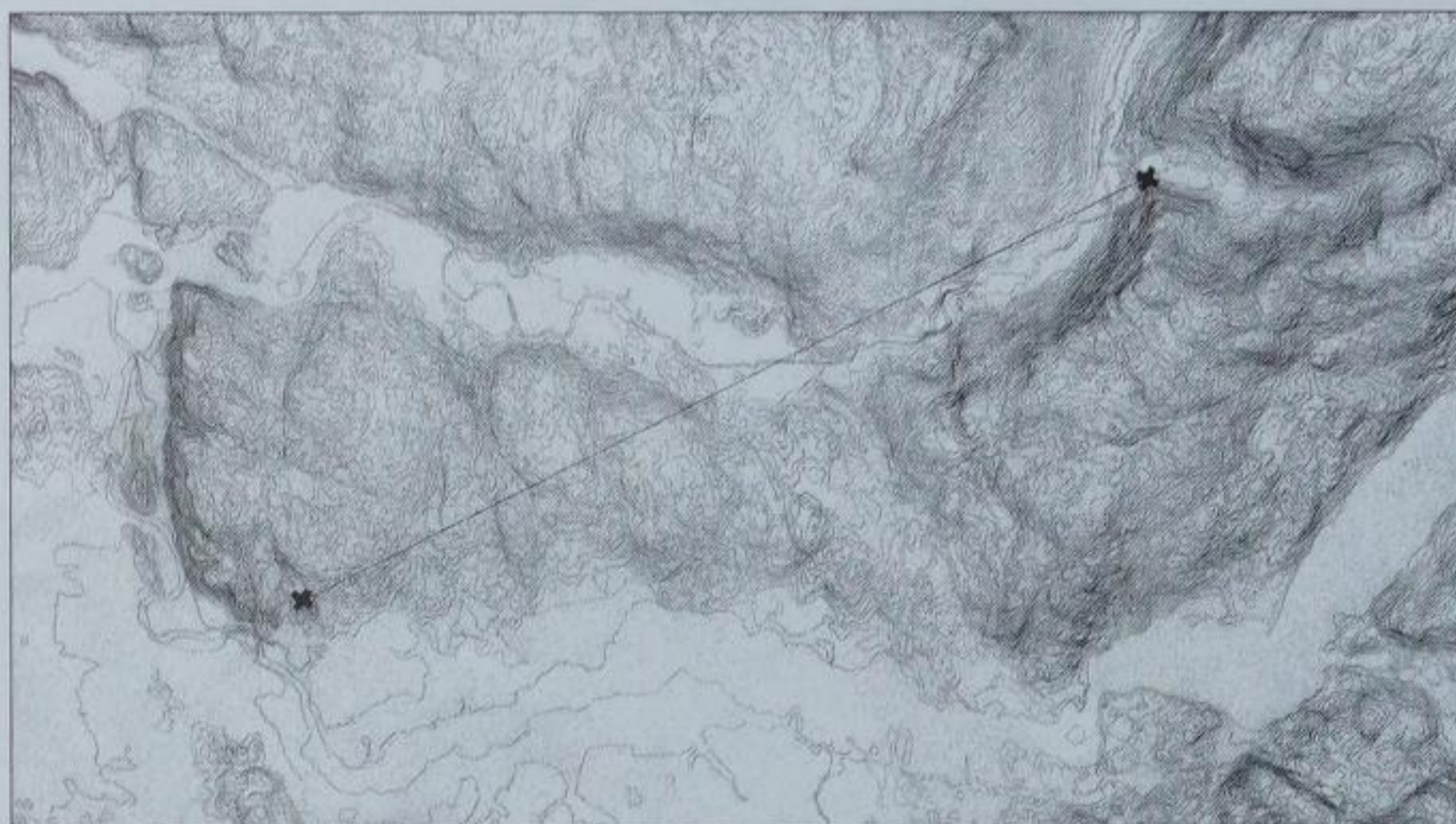
Glen Moidart The map shows the location and topography of the monitored site, and reveals the path the received signals are most likely to have taken from a local transmitter.
