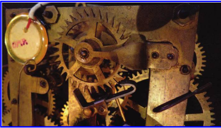
Fig. 4. Escapement detail. (Photo © Jay Needham)
