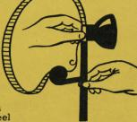
Locate the film-ring underneath film retainer near sprocket wheel
