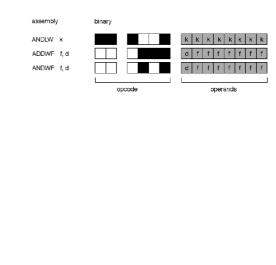
fig. 3b) assembly commands as binary patterns
