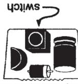
8. When removing Joe's switch, wires meet the circuit board. Heat contacts and remove switch.
