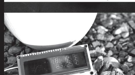
LCD display showing temperature inside the cooker
