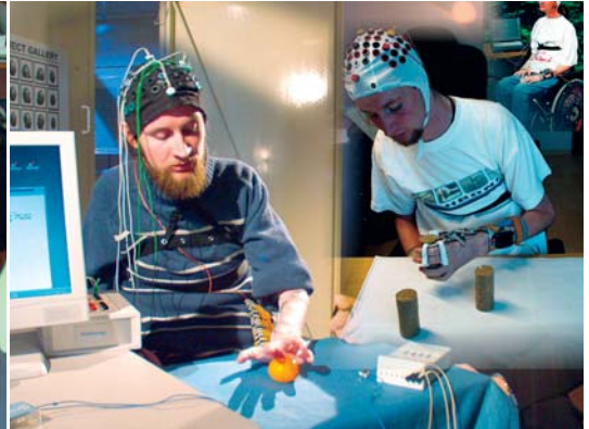
Tetraplegic patient with a BCI controlled orthosis and functional electrical stimulation grasp restoration, respectively
