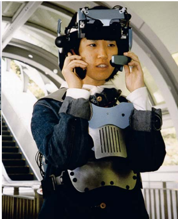
Dis-Armor, 2000: This instrument was used by high school students in Hiroshima. A microphone and two video cameras in the head piece transmit voice and images of the user's eyes to speakers and two LCD screens on his or her back. The piece also includes a rearview mirror, computer, and batteries, as well as wireless video transmission that allows pairs of users to wear each other's eyes and speak with each other's voices.
