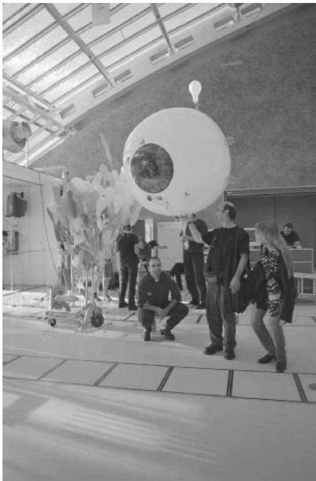
Fig. 6.3.8. Eric Paulos, Space Browser (1997). One of several small Internet-controlled telerobotic blimps with video and two-way audio that allows people to explore and interact within an installation space.
