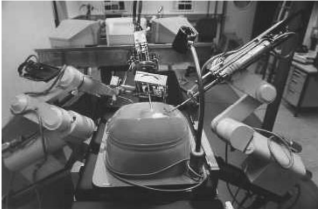
Fig. 6.1.8. ARTEMIS (Advanced Robot and Telemanipulator System for Minimal Invasive Surgery) experimental telesurgery system. Photo courtesy of Forschungszentrum Karlsruhe, ( http://www.iai.fzk.de/~artemis/arbeitsys/arbeitsysengl.html ).
