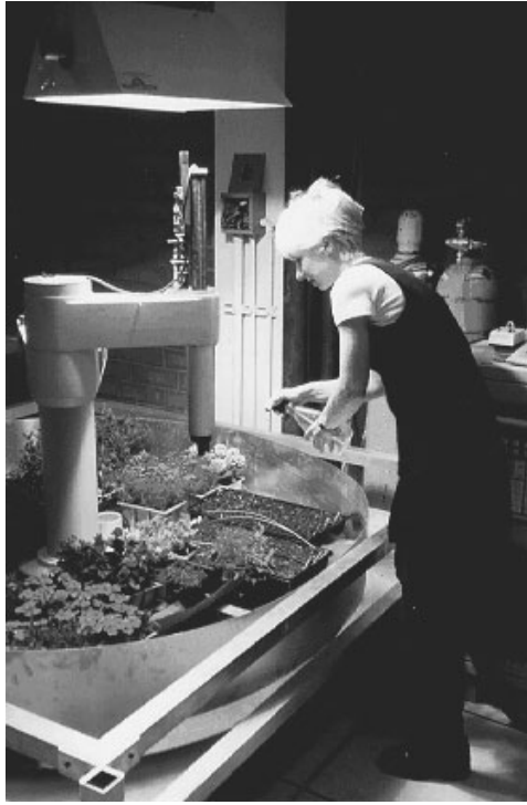
Fig. 6.3.5. Ken Goldberg, Telegarden . Web visitors can plant and tend seeds via a Web-controlled robot arm.
