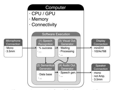
**Figure 5**. Systematic Analysis of the Computer as Sub-Element.
