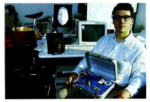
The hand is one of the most versatile of human instruments. but so far computers are blind to its expressiveness. One of the goals at the Media Lab is to make computers sensitive to the nuances of human gesture. Infrared LED's (light-emitting diodes) in this glove permit optical tracking. Just as a "mouse" is used to move a cursor around on a personal computer screen, this technique could provide a multiply-articulated "mouse" in three dimensions.
