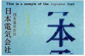
Anti-aliasing of Japanese kanji (here the relatively simple character for "tree") is even more effective than with Roman lettering because of the complexity of many ideographic symbols and the number of their horizontal elements, which are often poorly displayed on horizontally-scanned screens. (above)
