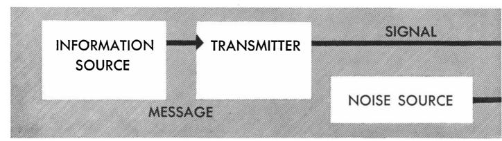
A COMMUNICATION SYSTEM may be reduced to these fundamental elements. In telephony the signal is
