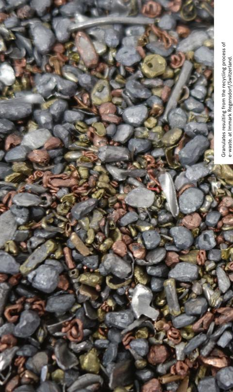
Granulates resulting from the recycling process of e-waste, at Immark Regensdorf/Switzerland. COPYRIGHT (C) 2015 Research team "Times of Waste"
