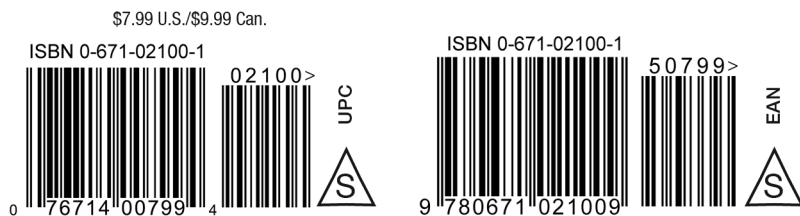
FIGURE 8 UPC and EAN product codes for a book intended for sale in nonbook outlets, printed on the outside back and inside front covers, respectively.
