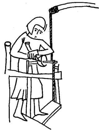
Pole lathe (French fourteenth-century MS).
