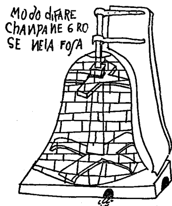
Ghiberti: model for bell-making.
