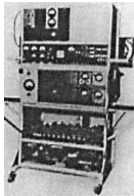
Figure 15 The final form of the analog computer in Peenemünde, 1943
