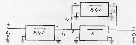
Fig. 5—Generalized circuit for operational computation.
