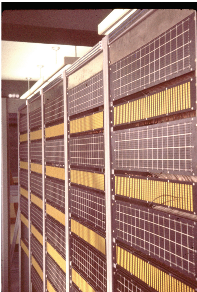
Fig. 2.8. Patch panel components of the Tobermory Perceptron. Image from Frank Rosenblatt's camera, courtesy of William Mutch.
