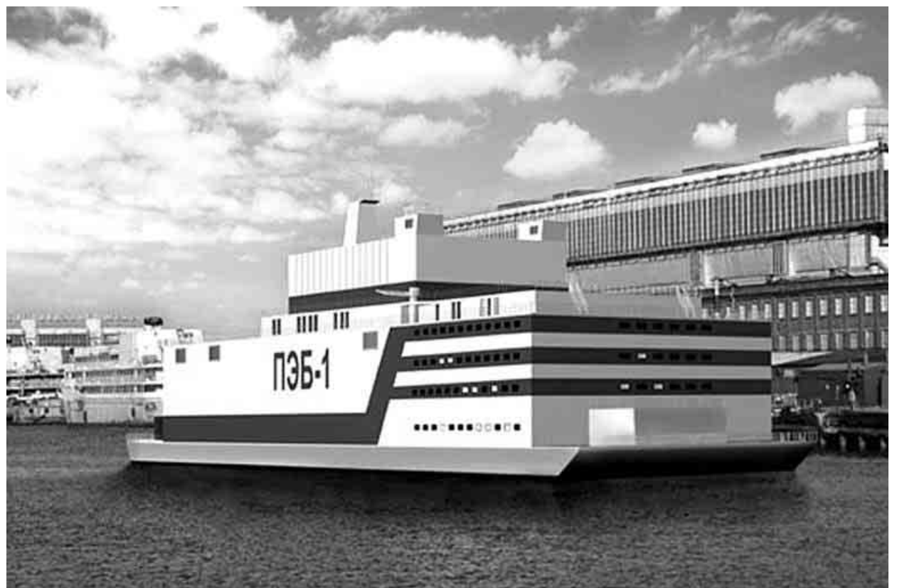
ATES MM on Sevmasht : nuclear station of small capacity (ATES MM) on the basis of floating power generating plant reactor unit KLT-40S (reactors of such type have been successfully used on nuclear ice-breakers for more than 35 years).
