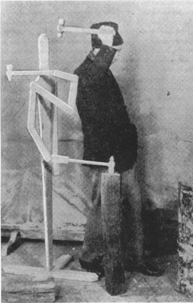
79 "Training in hammering," from "The Russian Central Institute of Work and Its Methods and Means for Training Workers," Management Engineering: The Journal of Production (New York) 4, no. 4 (April 1923), 243. This photograph documents a typical training exercise at TsIT—in this case, a worker being instructed by a mannikin in the art of hammering. The mannikin's two left arms demonstrate the correct (i.e., the most efficient) posture of the arm relative to the body at the start and conclusion of its swing. Mannikins, templates, jigs, training frames, and photo-cyclograms are often used at TsIT in the instruction of unskilled workers in correct body postures and work-motions. Photograph courtesy of Wirtz Labor Library, Washington, D.C.
