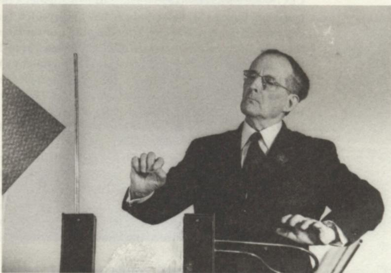
fig 2.9 Leon Theremin playing on the fingerboard Theremin at the Acoustical Laboratory at Moscow Conservatory, c. 1965. The right hand adjusts the loudness by means of a special lever equipped with a set of buttons to control the timbre by means of additive synthesis. TCA.
