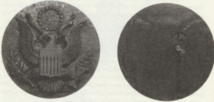
fig 2.29 The Great Seal wall plaque. Left: front view of the carving. Right: cutaway view showing concealed trench containing Theremin's passive resonant cavity transmitter. Courtesy of thespymuseum.com, and H. Keight Melton, *The Ultimate Spy Book* (New York: DK Publishing, 1996).
