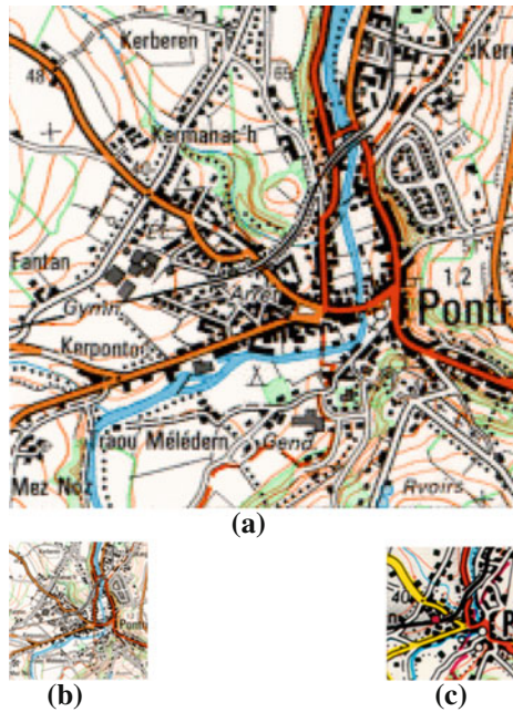
Fig. H.15 a Part of a map at 1/25000 scale. b A 16-fold reduction of the map. c Cartographic generalization of the map at the 1/100 000 scale. By comparing b and c the differences between simply reducing and generalizing are clearly apparent
