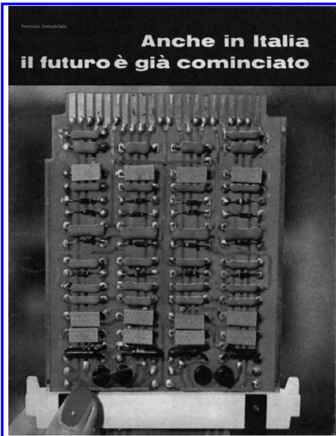
Illustration of an integrated circuit from the first computer produced in Italy, the Olivetti ELEA 9003. From Epoca (1959).
