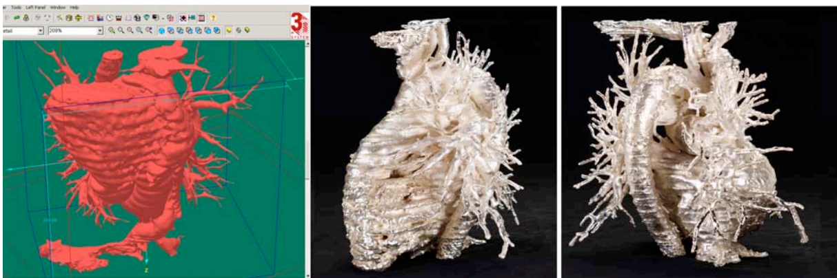
Heart (2004) MRi data of healthy human heart reconstructed for rapid prototyping. Two angles of the resulting rapid prototype, silver plated.
