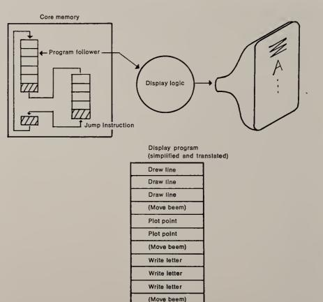
A high-power display ordinarily, these days, uses the core memory of a small general-purpose computer. Both can use the same memory intermittently, each program unbeknownst to the other.
